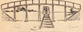
WAGON ROAD CROSSING. [The manner in which a country road will be made to cross the line of the electric railway by means of a wooden bridge. It is estimated that about 250 of these will be required between Chicago and St. Louis.]
